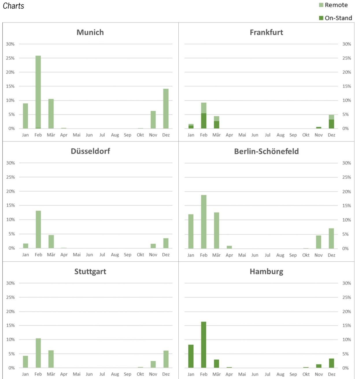
Fig. 4: Share of IFR departures 2017 requiring aircraft de-icing on stand (dark green) and remotely (light green)
