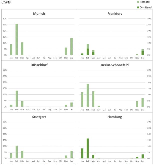
Fig. 4: Share of IFR departures 2017 requiring aircraft de-icing on stand (dark green) and remotely (light green)
