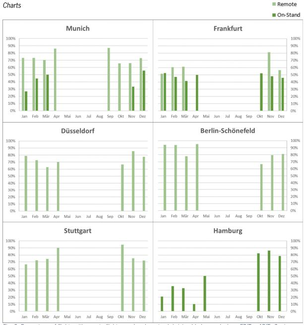
Fig. 9: Percentage of flights with remote (light green) and on-stand de-icing (dark green) where  $EDIT = ADIT \pm 3 \text{ min}$
