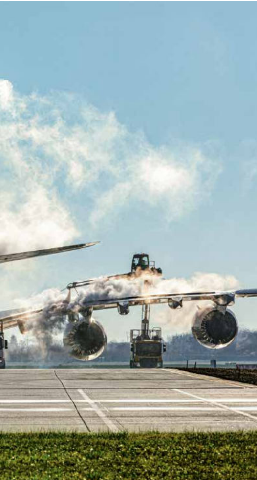
Special vehicles known as «polar bears» spray the aircraft with de-icer.
