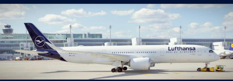
With our conventional and towbarless tractors we are able to move all aircraft currently approved for flight operations. By firmly clamping the front landing gear, the towbarless tractors can execute towing operations considerably faster than conventional towing tractors. In addition, towbarless tractors offer greater safety as the possibility of a broken towbar can be ruled out.
