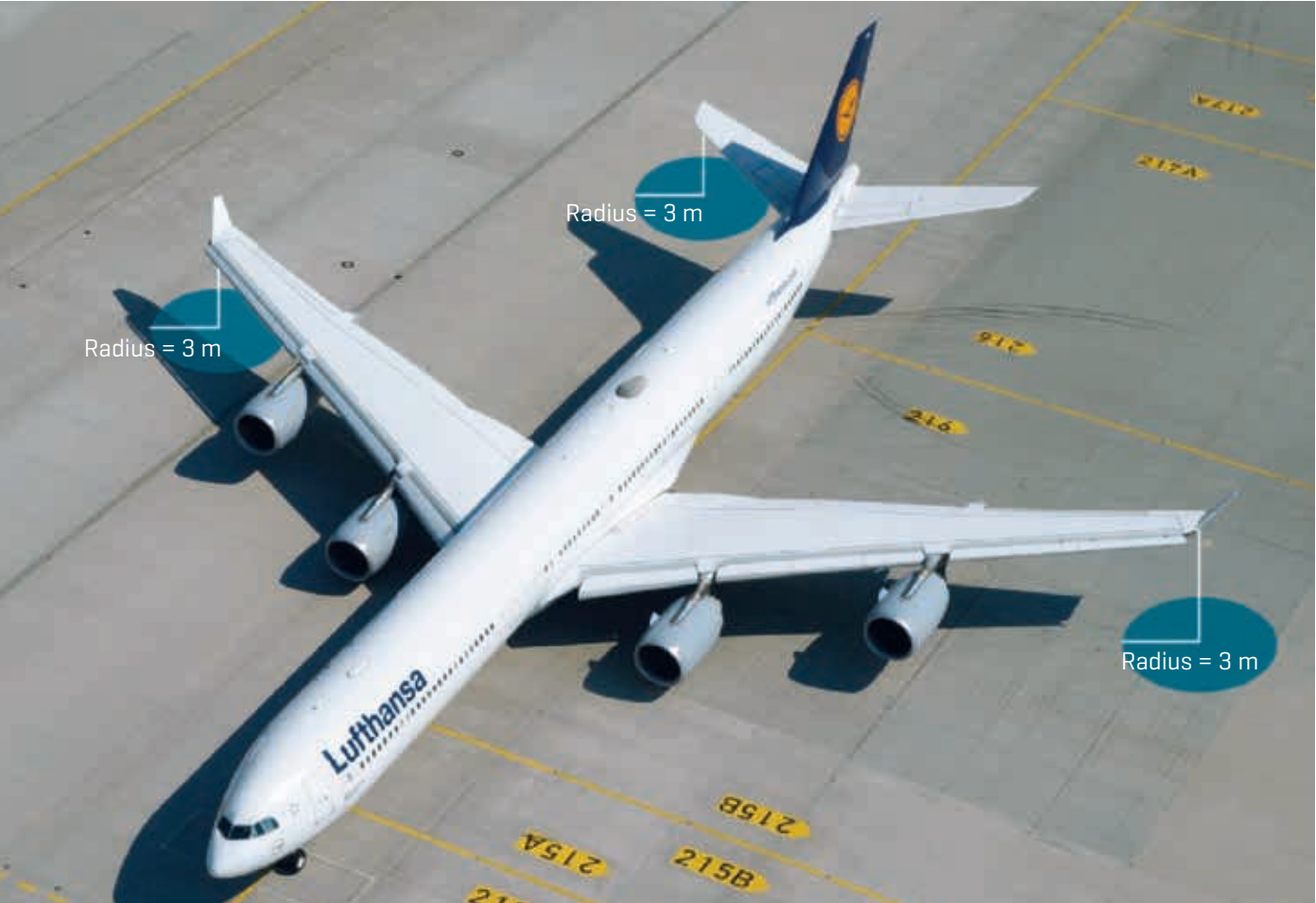
There is an additional tank vent on the right elevator on aircraft with a trim tank in the elevator [e.g. Airbus A330, A340, A380, or Boeing 747].
